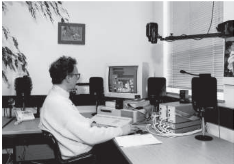
A Medusa workstation equipped with multiple cameras, speakers and microphones. Note the ATM network switches in the lower right, just under the video bricks.
