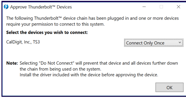
Fig. 6: When a malicious Thunderbolt device is attached, Windows prompts for access without a description of what rights are being requested. Users cannot make an informed decision whether to enable a device.
