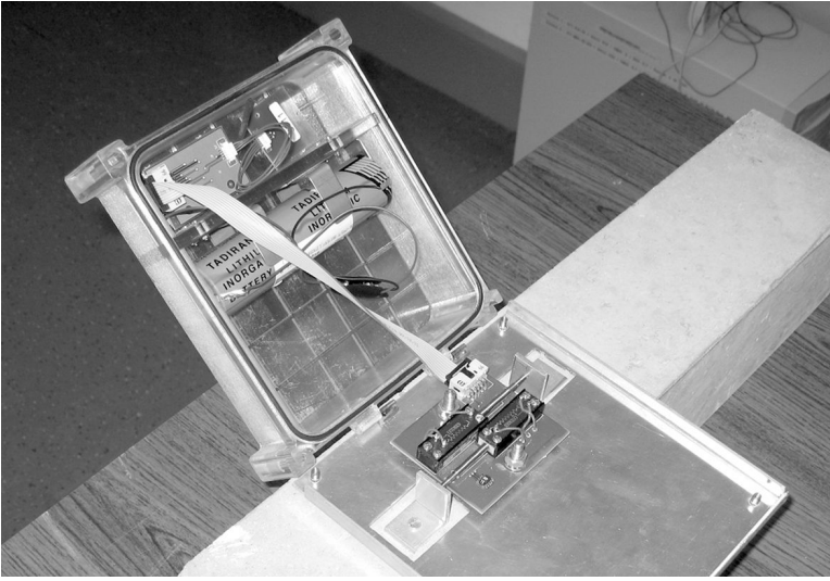
Figure 7: We designed and built an LPDT sensor box with two Linear Potentiometer Displacement Transducers (LPDTs) to measure crack width to a resolution of 10\ \mu\text{m} . The box is fastened to the concrete bar below and the potentiometer cursors are attached, with brackets, to either side of the crack that lies under the box. One of them measures the crack width and the other the thermal expansion of the concrete, for calibration. (Cfr. principle 14.)
