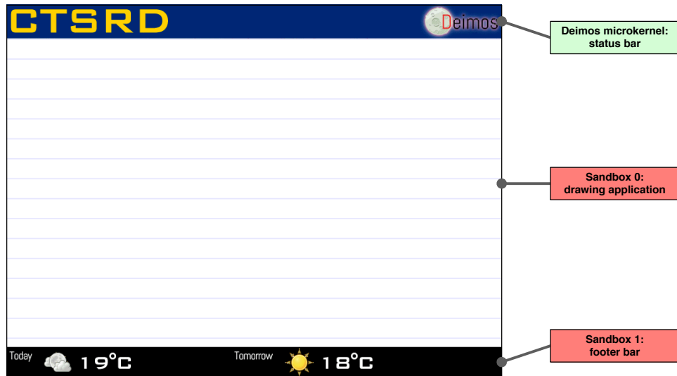
Figure 4.1: The Deimos touchscreen interface
